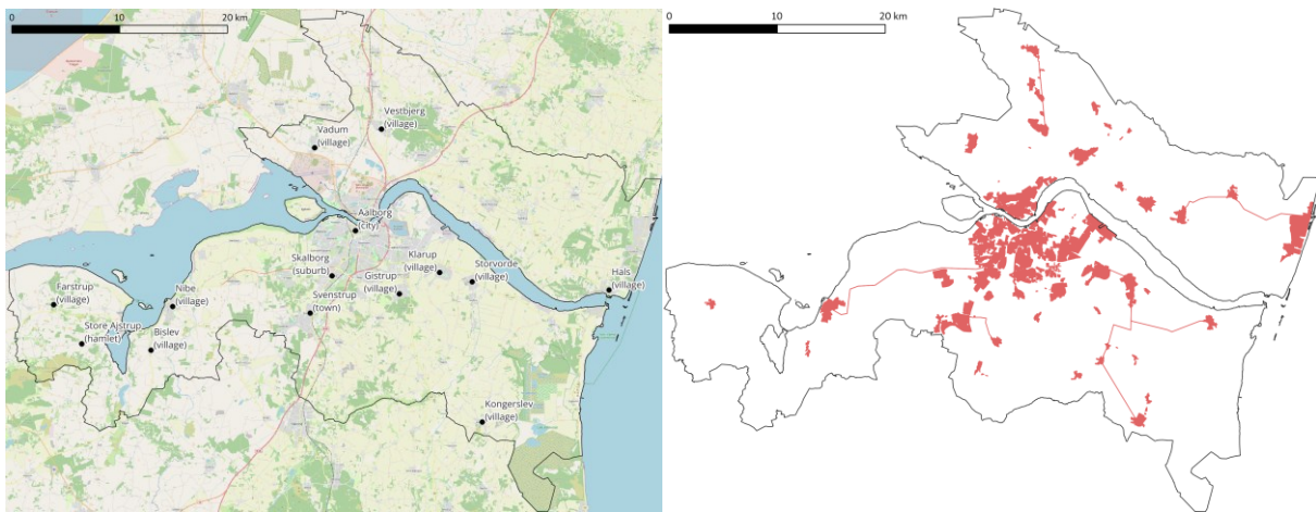
Figure 21. Map of Aalborg area (left panel) and of the existing district heating infrastructure (right panel). It can be seen that the connected area basically covers the entire urban area.
