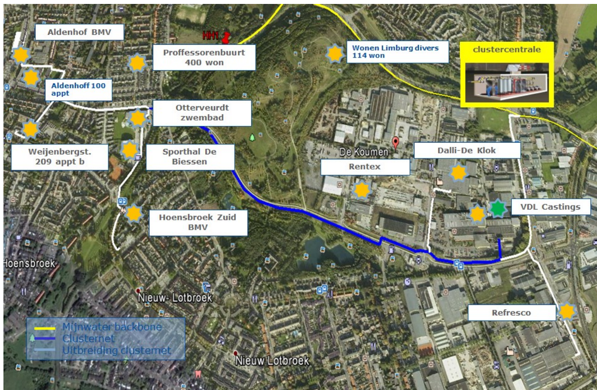
Figure 20. Some of the identified prosumers for cluster D. Some of them are already connected (VDL foundry and Otterveurdt swimming pool were connected as part of the LIFE4HeatRecovery project). Similar maps have been developed by Mijnwater for the other network clusters and the surrounding areas.
