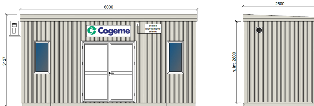
Figure 5 – heat exchanger kit container.
